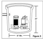
If the AC/ DC Sump Pump is to be used as a backup for an electrical primary pump it is important to maintain a minimum water level of 6 inches in the sump when measured from the bottom of the AC/ DC Sump Pump. The water is needed to allow the AC/ DC Sump Pump to go through its 24-hour testing cycle. You will need to adjust the off level of the Electrical Primary Pump to turn off at the minimum water level of 6 inches as shown in Figure 4.
